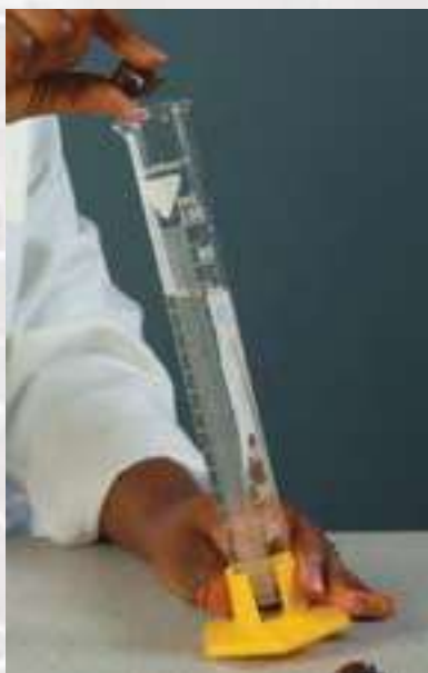
The formula method for determining density: After finding the mass of an object, measure its volume by water displacement.
